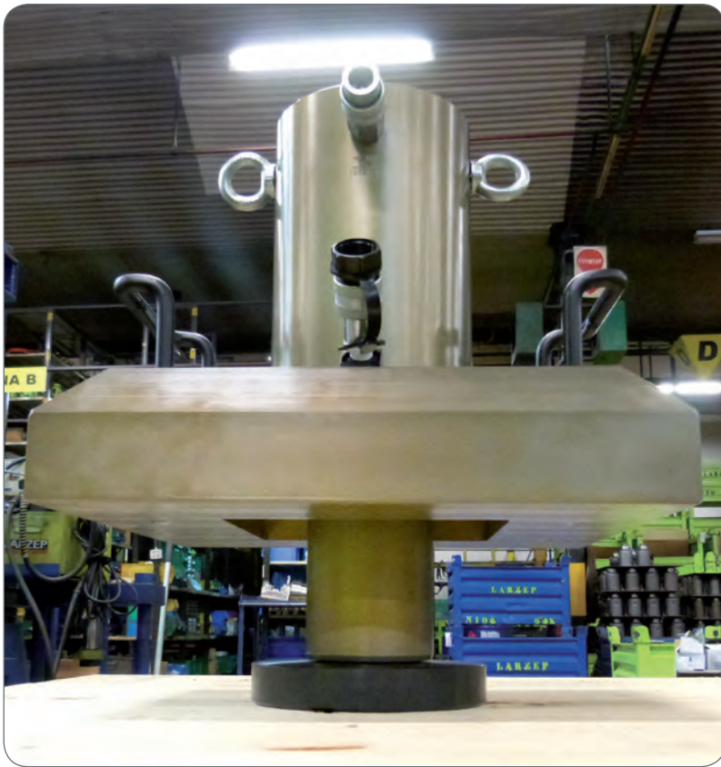
Step by step aluminium cylinders. Stage lifting.
