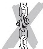
The unit itself must never be used as a means for attaching ropes, chains or belts.
