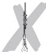
Do not tie knots in the chain or connect it by using bolts, screws, screw drivers or similar for attaching the unit. Chains permanently fitted in the load lifting attachment must not be repaired. Do not pull the chain over edges.
