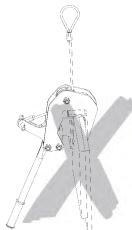
It is forbidden to apply lateral tensile forces to the load lifting attachment.
